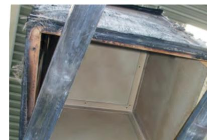
The FIRE SHELTER was able to keep the interior temperature below 60°C for 2 hours. This ensures a correct functioning of the equipment during emergencies. Our solutions were tested several times by independent bodies, the results of which are available on request.
