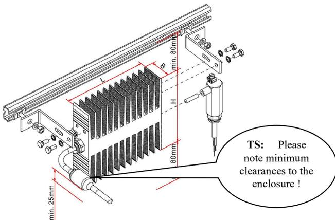
The brackets in zinc coated steel and fixing bolts illustrated above are included with the heater. Furthermore, a short threaded rod for mounting the TAE thermostat on the heater is supplied with the TAE.
