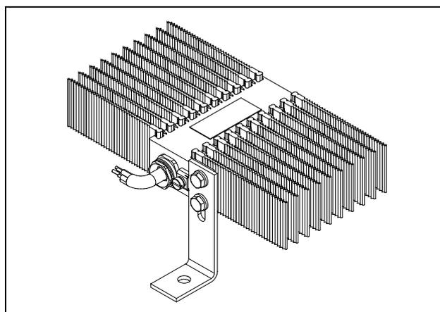
The mounting bracket can be installed on either end of the block.
