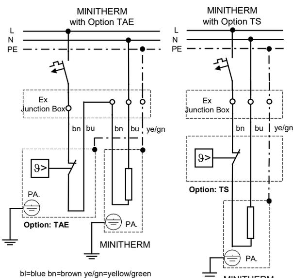
Connection cable: silicone cable, notch and oil resistant,  $3 \times 1,5 \text{ mm}^2$ , 1m long. Other lengths available upon request (at an extra charge).
